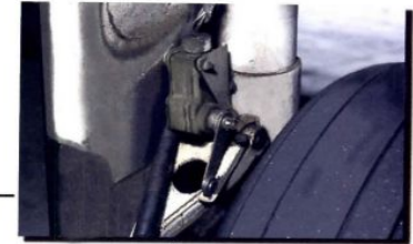
Figure 11-49. This safety switch is located on the left main gear. While some safety switches prevent gear retraction by opening the electrical circuit, some keep the gear switch inside the cockpit from moving.
